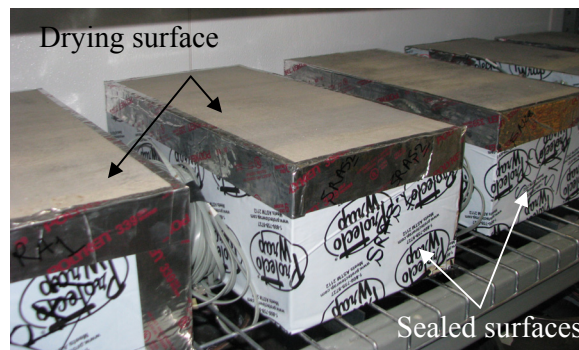
Figure 2: Slab geometry with one-sided drying
