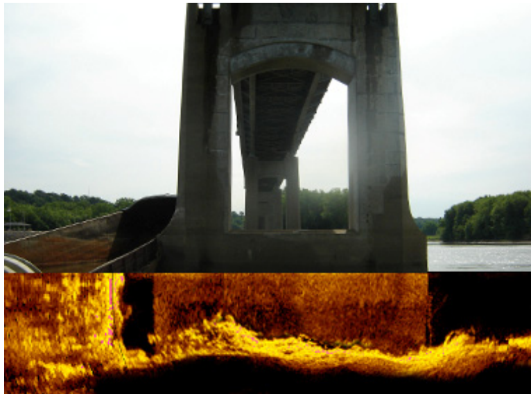
Figure 27. Sector-scanning sonar image of submerged barge at upstream nose of pier.
