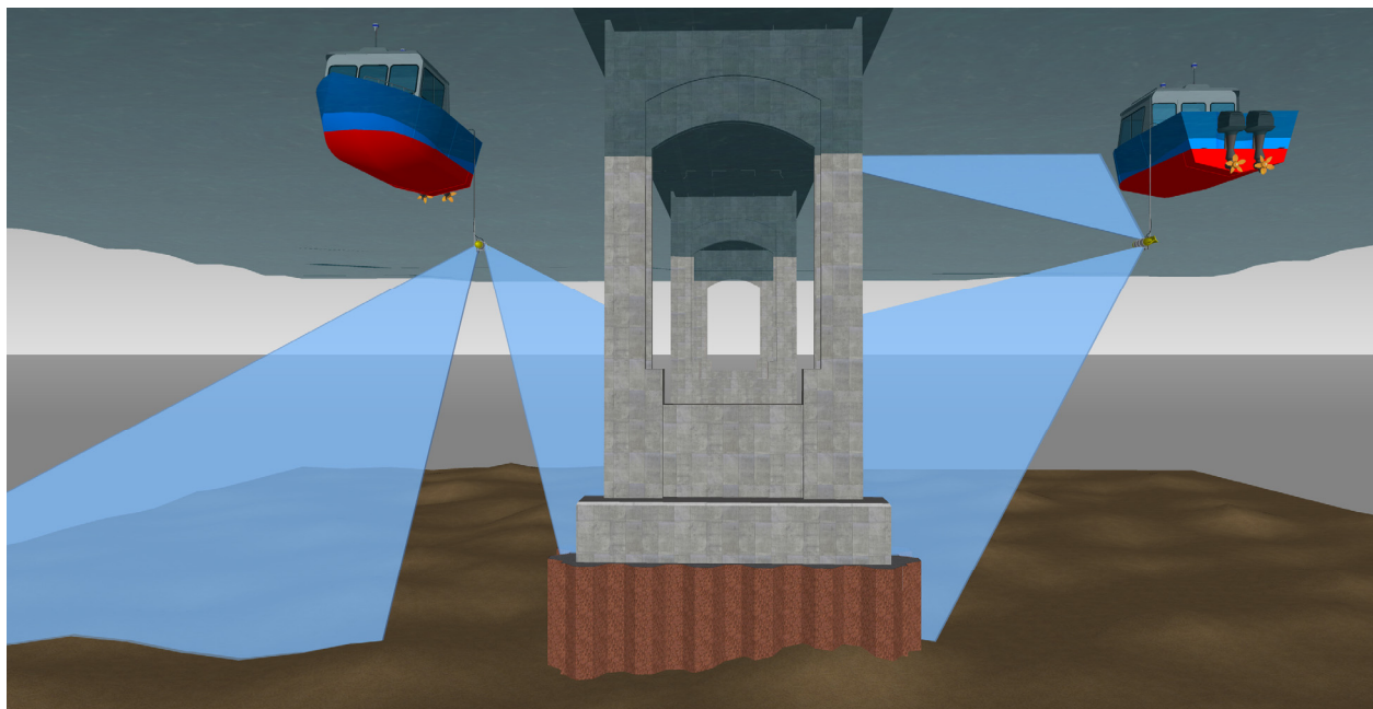
Figure 16. Side-scan sonar mounting positions for structural imaging (right) and bottom scanning (left).
