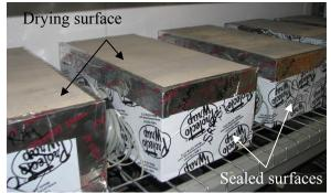
Figure 2: Slab geometry with one-sided drying
