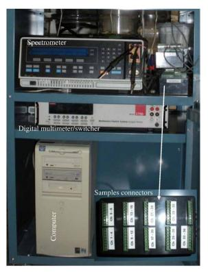
Fig. 2. Components of the system.
