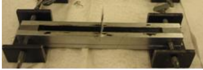
Figure 2. SENB specimen mold.
