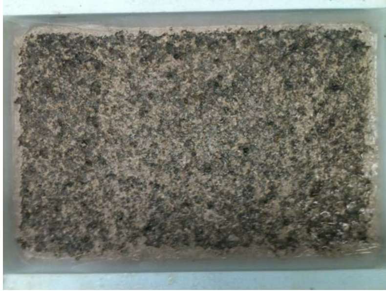
Figure 2: VaDOT exposure for Mix #13 50%LA 50%SG120 0.42w/c at 25cycles where finer scaling is observed
