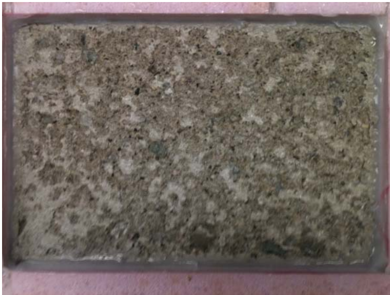
Figure 1: ASTM exposure for Mix #13 50%LA 50%SG120 0.42w/c at 25cycles where coarser scaling is observed
