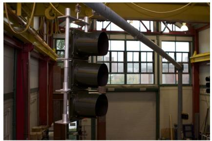
FIGURE 3 Signal head vibration mitigation devices tested at UConn.
