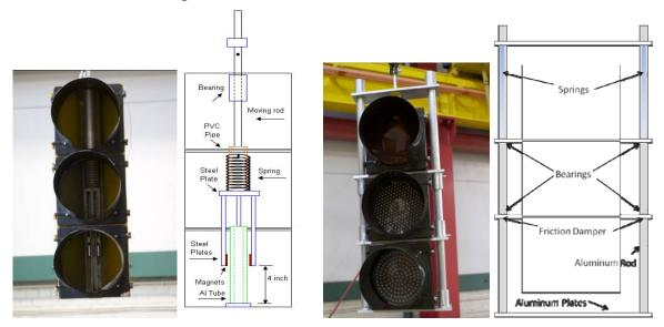
FIGURE 2 Signal head vibration mitigation devices tested at UConn.
