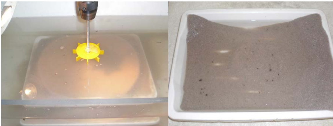
Figure 12 Physical modeling of impeller erosion mechanism
