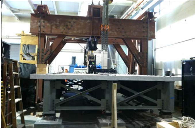
Fig. 1 View of three-girder test set-up with composite concrete deck
