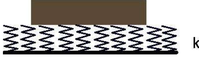
Figure 2.1 Slab on Winkler foundation [6]
