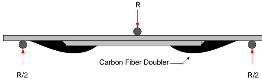
**Figure 4: Fatigue Specimen with Composite Application**
