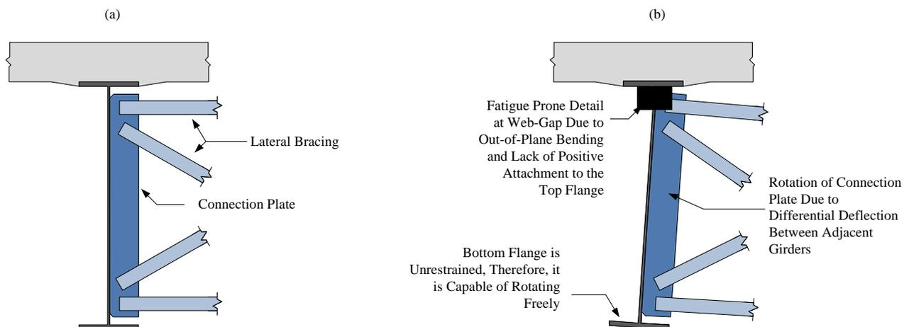
**Figure 1: (a) Girder Cross-Section before Differential Displacement
