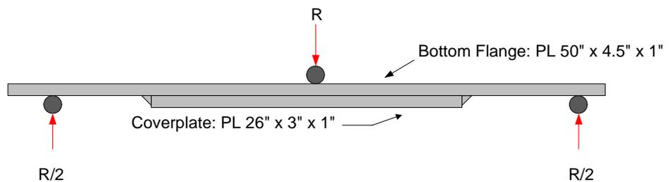
**Figure 3: Fatigue Specimen in Three-Pt. Bending**
