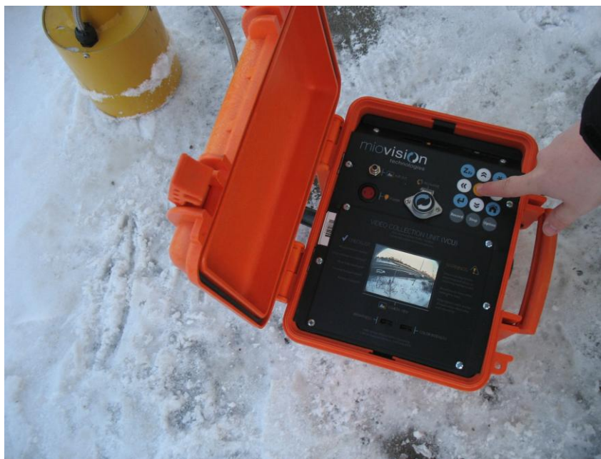
Figure 35. Miovision VCU with Video Display
