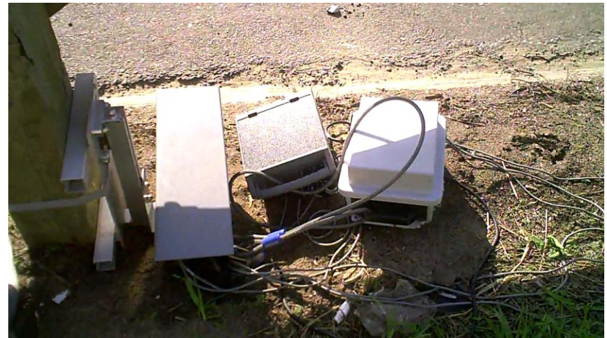
AxleLight, PEEK ADR 1000 and battery module.
