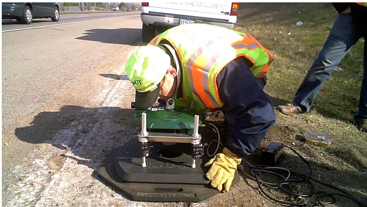
Figure 26. TIRTL Setup--Aiming With Scope
