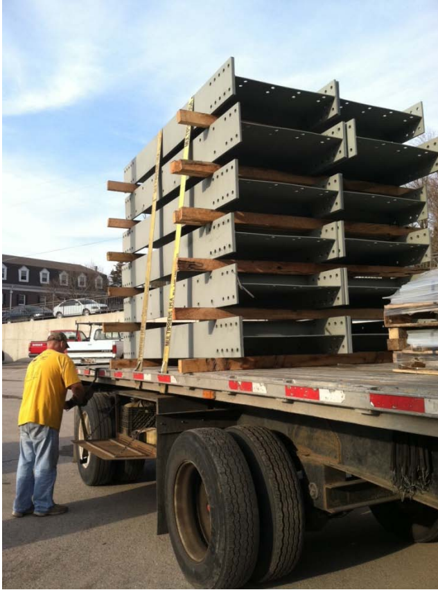
Fig. 1. Shipment of girders from CTIW received at the KU Structures Lab for use in 30 ft. girder test set-up
