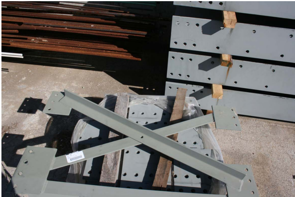
Fig. 3. View of one of the typical cross-frames to be used in the bridge test set-up
