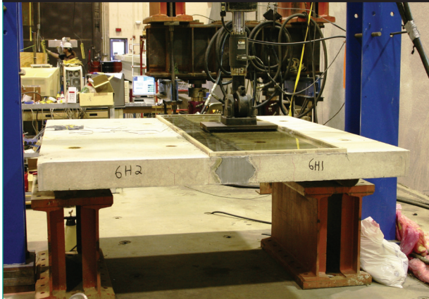
Figure 3. Field-cast UHPC longitudinal connection cyclic test setup.
