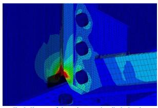
Fig. 9. Close-up of the web gap region displaying the distribution of maximum principal stresses
