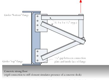
Fig. 4. Cross-section chematic of the test set-up for the 9' girder specimens
