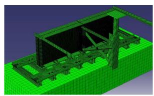
Fig. 7. Overall view of the finite element model for the 9' specimens
