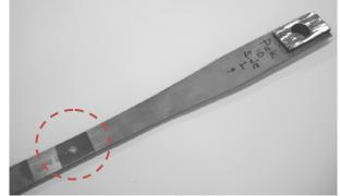
Fig. 11. View of the specimen with brittle coating applied around hole (circled region)
