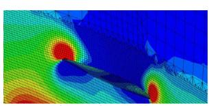
Fig. 8. View of the back of the web, showing the crack opening under distortion-induced fatigue
