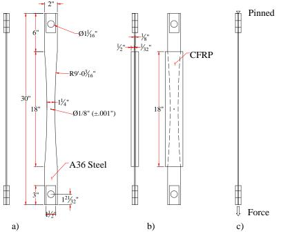
Fig. 14. Schematic of the tensile fatigue specimens outfitted with CFRP doublers
