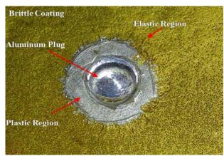
Fig. 13. Close view of the PICK-treated hole with brittle coating flaked-off in region of plasticity
