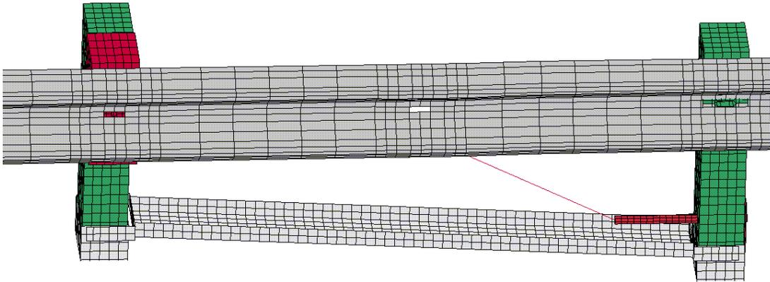
Figure 1. Old Terminal Model used for MGS Simulations
