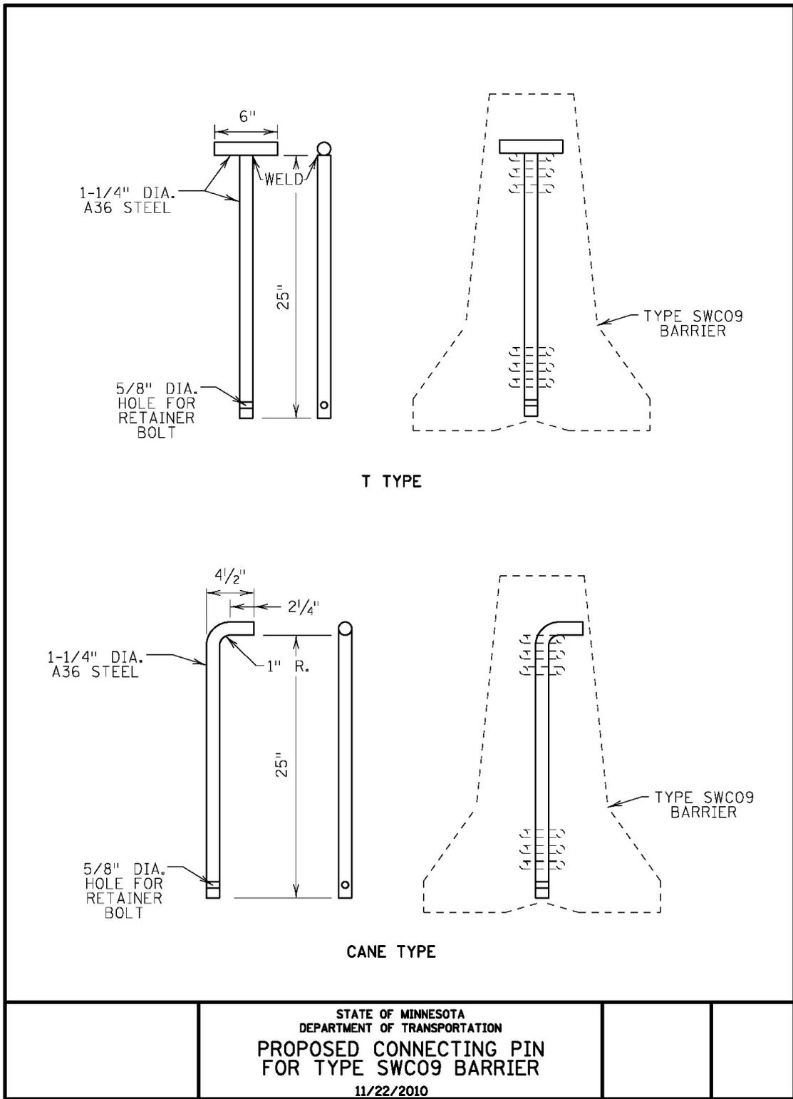
Figure 2. Proposed F-shape Barrier Pin Designs
