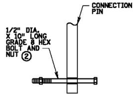
RETAINER BOLT AND NUT DETAIL
