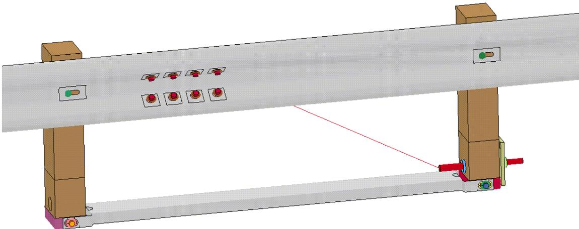
Figure 3. New Terminal Model used for MGS Simulations – mesh turned off
