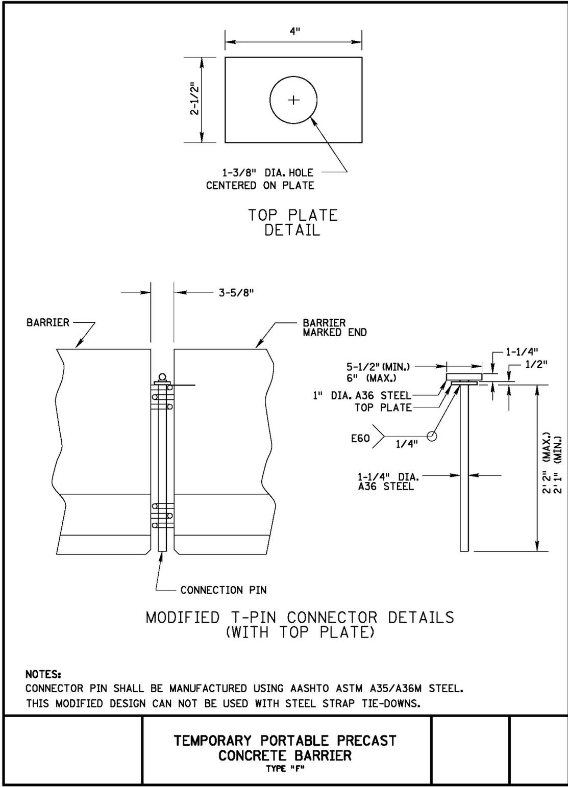
Figure 5. Final MnDOT Connection Pin Design
