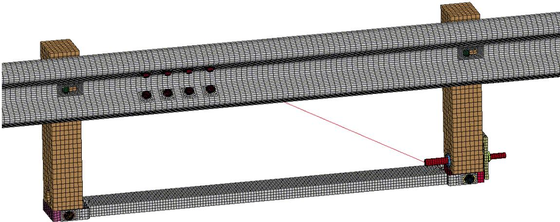
Figure 2. New Terminal Model used for MGS Simulations
