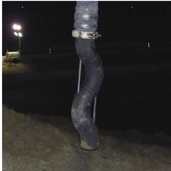
Fig. 5.8 – “S-Hook” fitted to the end of the pump discharge hose used to limit air loss through the pump.
