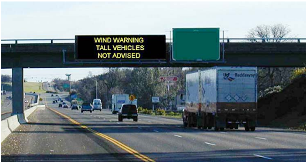
Figure 17: Example of Dynamic Message Sign
