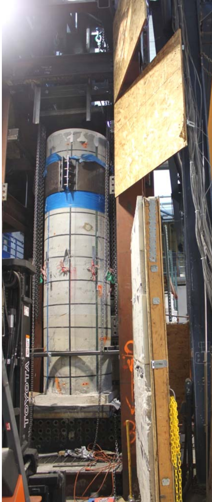
Figure 11. Test setup for the 12 ft high – 3 ft diameter columns
