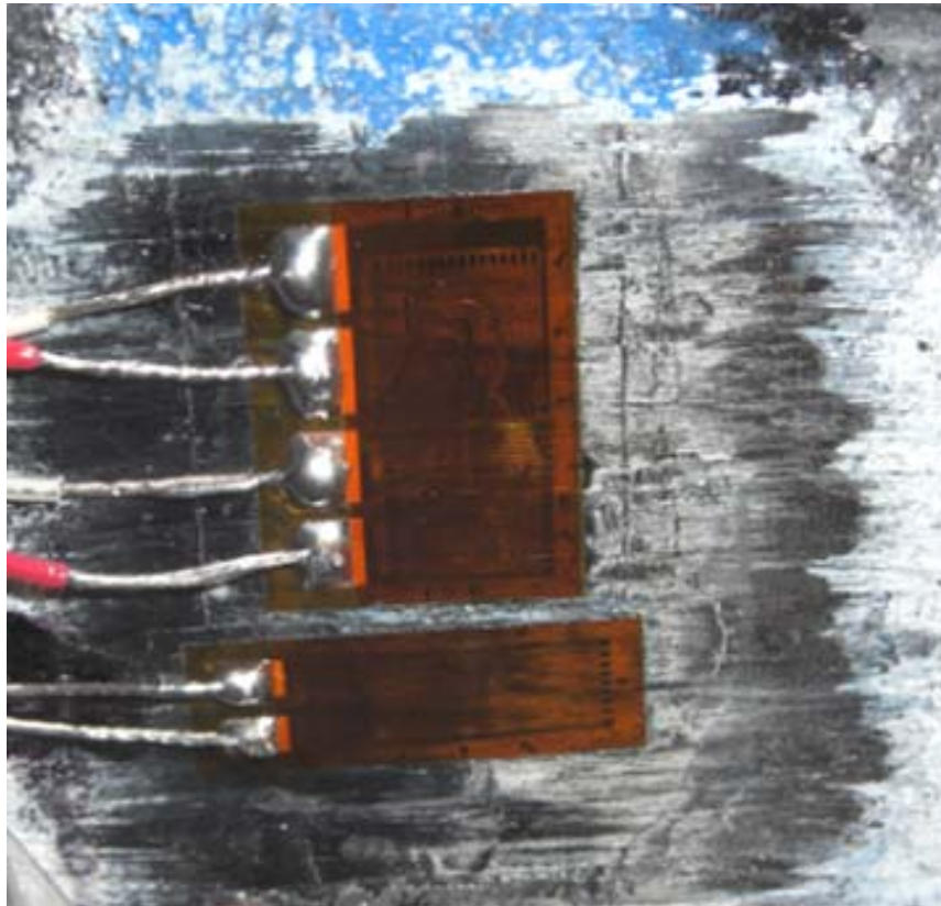
Figures 7. Strain gauge arrangement and close up of strain gauges
