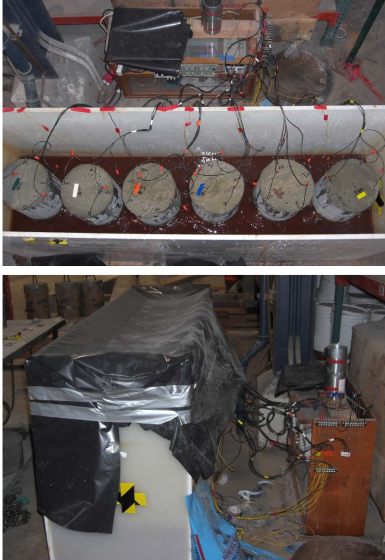
Figure 2. Corrosion system for small-scale steel reinforced columns
