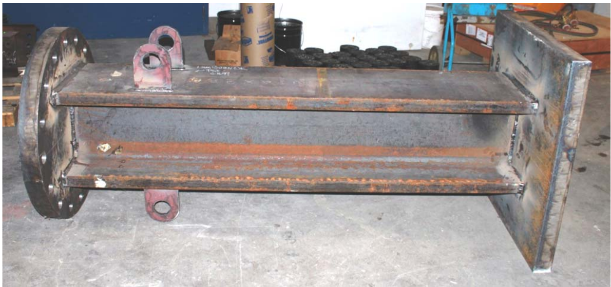
Figure 9. Column connector to actuator (W 14 x 283 steel column)
