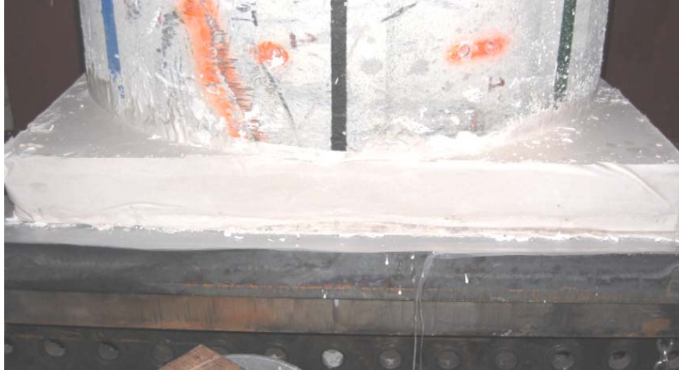
Figure 6. Bottom column cap (thickness between bottom of column and steel plate 2in.)
