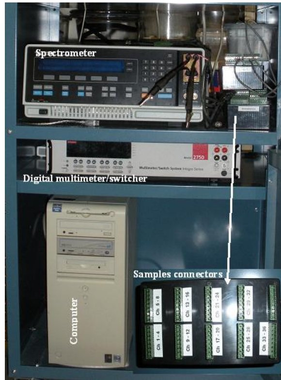
Figure 4: A view of the new designed system (AEMS) to assess electrical properties in concrete
