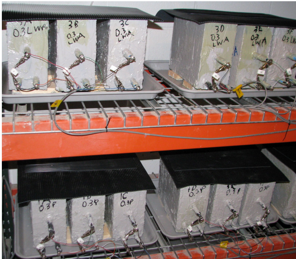
Figure 8: Samples Prepared According to ASTM G109
