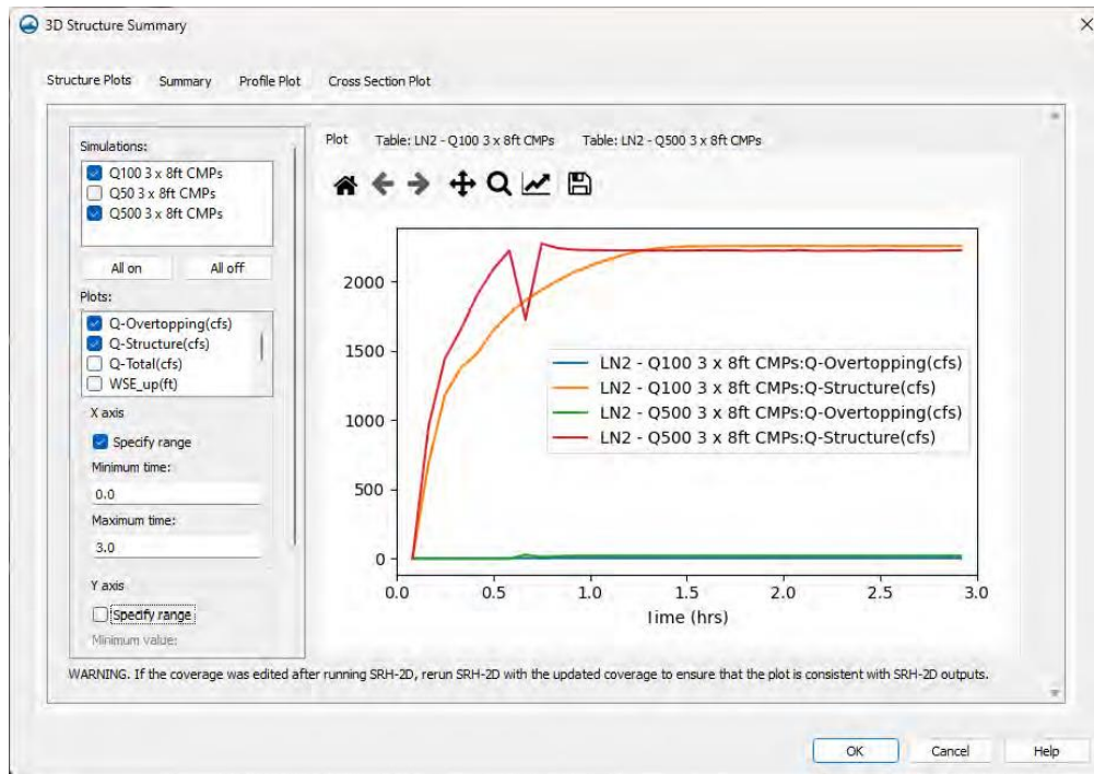
Figure 2 – Time series plot of flow going through multi-barrel culvert system with 3D structures tool.
