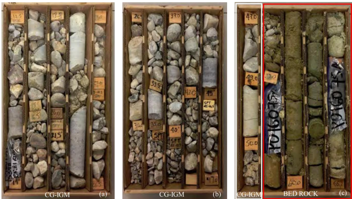
Figure 5.2. SH-28 Lemhi River Bridge Project Core Samples Indicate a) CG-IGM Starting From 12.5 ft, b) CG-IGM, and c) CG-IGM Terminated at 50 ft Overlaying the Bedrock.
