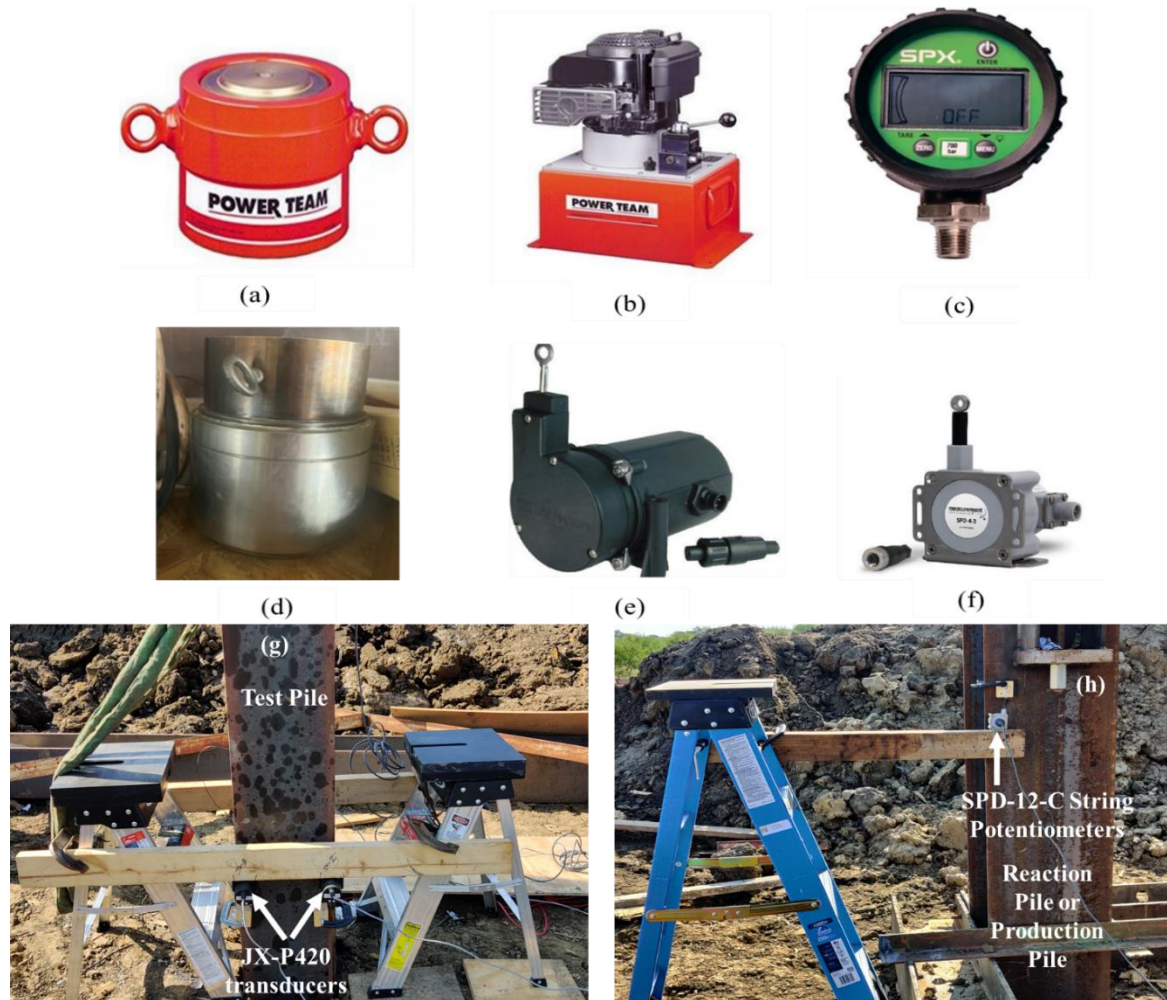
Figure 3.9. Instruments and Equipment Used in the SLT: a) Hydraulic Jack, b) Hydraulic Pump, c) Digital Pressure Reading, d) Load Cell, e) Linear Position Transducers to Measure Test Pile Displacement, f) String Potentiometer to Measure the Upward Displacement of Reaction Piles, g) Linear Position Transducers on Reference Beams Supported by Two Ladders at the Test Pile, and h) String Potentiometer on Wooden Beam Supported by the Ladder at the Reaction or Production Pile.
