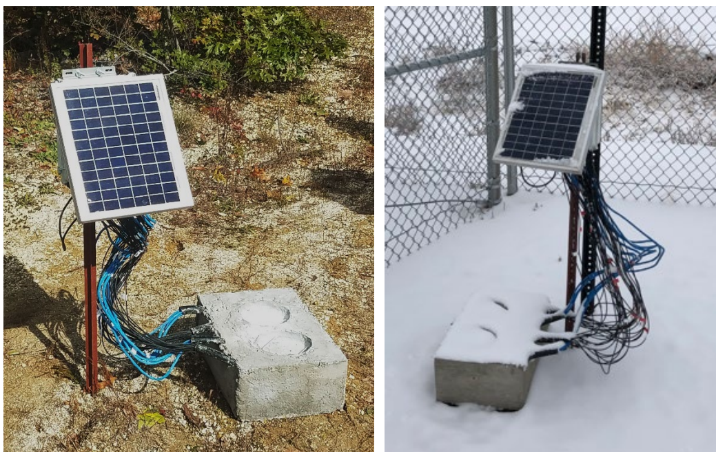
Fig. 3. Installed field samples, with the instrumentation box and solar panel set up for data collection.
