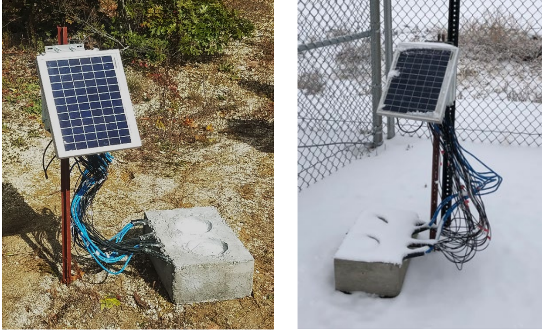
Figure 3: Installed mortar samples in the field, with the instrumentation box and solar panel set up for data collection.
