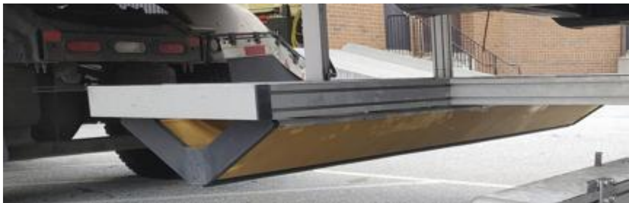
Figure 2. Installed 3D GPR antenna.
