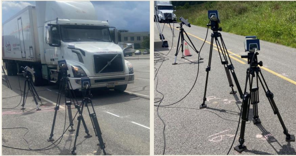
Figure 8. LDV setup on the Surface Street section (left) and Rural Roadway section (right).
