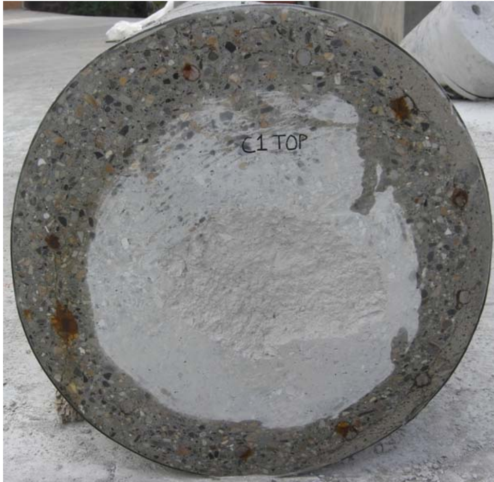
Figure 7. Corrosion of vertical steel reinforcing bars at the top of full-scale column C1.
