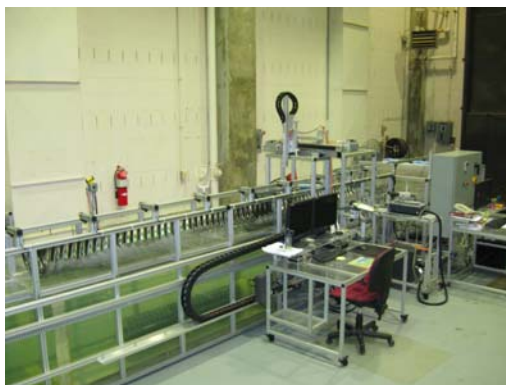
Figure 1: New corrugated pipe (diameter 18" with 2.66"x0.5" corrugations) installed in the culvert flume.
