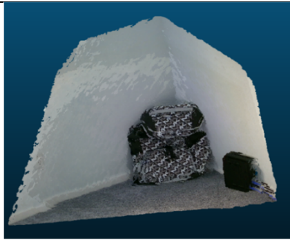
Figure 8. A sample 3D mesh model created by a short video from the RGB-D camera
