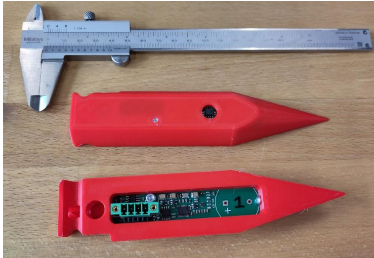
Figure 1: Pressure sensors mounted in their casing.
