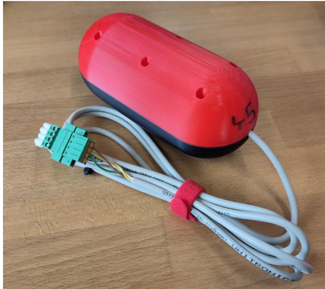
Figure 3: Geophone enclosed and with cable.
