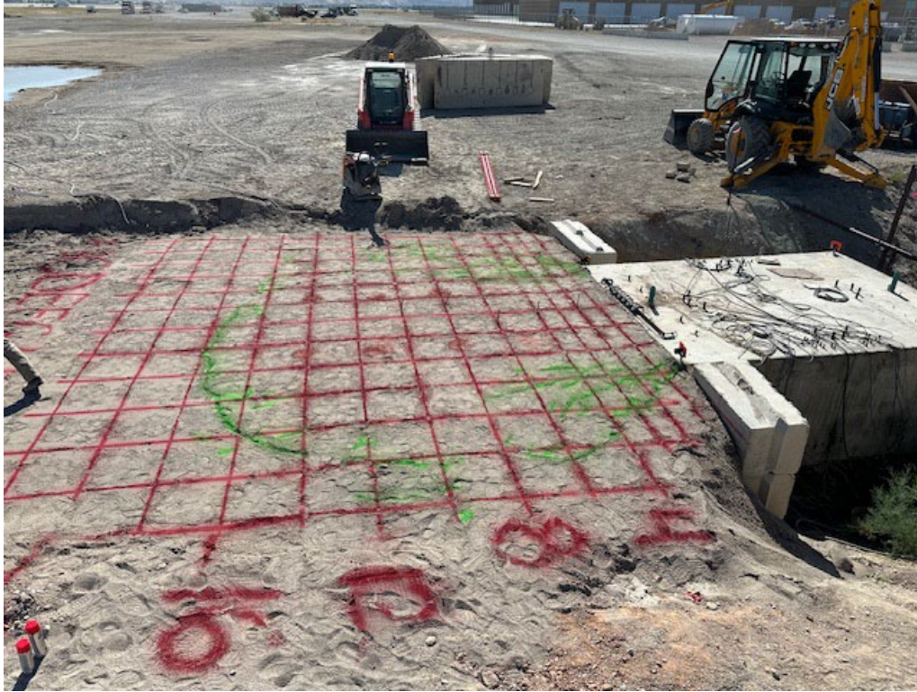
Fig. 4 Photograph of backfill with red grid for no skew ( \Theta = 0^\circ ) test along with failure surface daylighting (green spray paint) with three-dimensional geometry.
