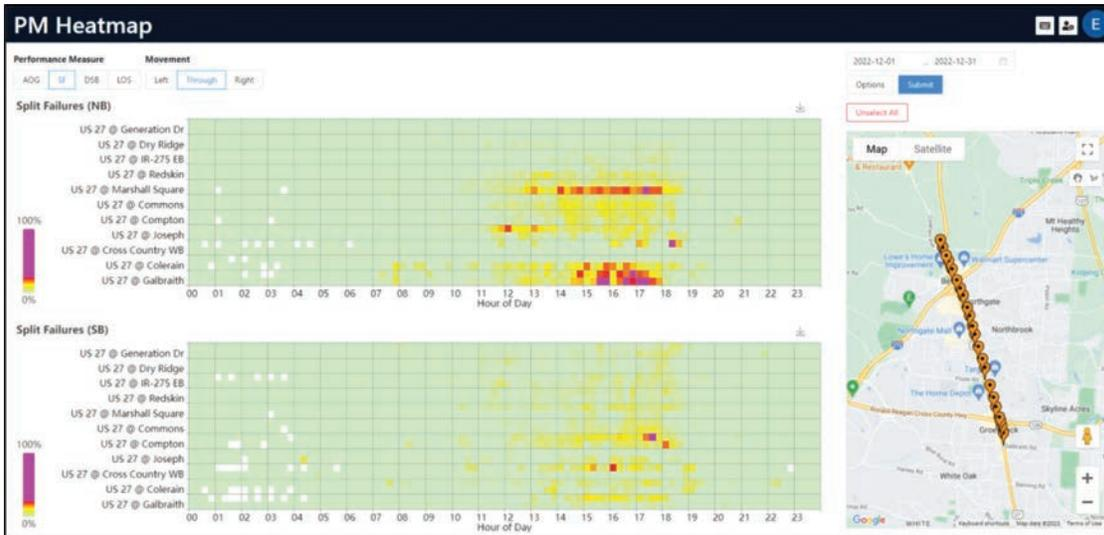
Figure 13.4 PM Heatmap web dashboard showing SF results for a 22-intersection corridor in Cincinnati, OH.
