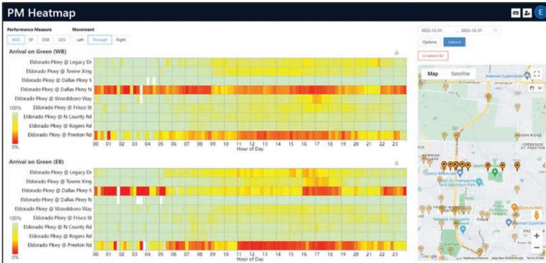
Figure 13.3 PM Heatmap web dashboard showing AOG results for a 9-intersection corridor in Frisco, TX.
