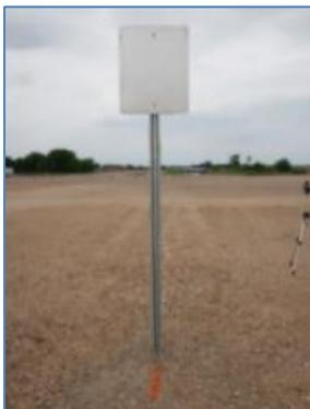
The initial objective was to evaluate the U-Channel Sign Support System according to the complete MASH TL-3 matrix. However, only MASH Test 3-62 was performed on the system due to excessive vehicle deformation observed during the crash test. The U-Channel Sign Support system did not meet the performance criteria for MASH tl-3 Support structures.
