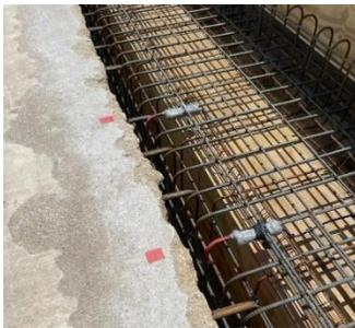
This research project installed strain gauges in a test installation of a concrete bridge rail that was constructed on a concrete bridge deck. The strain gauges were attached to the steel reinforcement of the barrier and the deck to obtain loads during vehicle impact. The bridge rail was impacted under MASH Test 4-12 impact conditions with a 22,000-lb single unit truck. The data collected from the test provides useful loading information for bridge rail and deck design.
