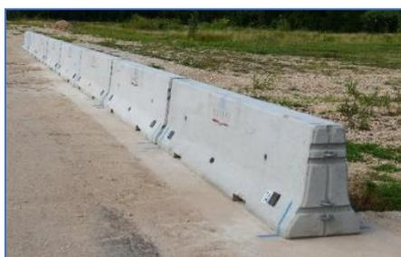
The objective of this research was to evaluate the MASH TL-3 performance of a 32-inch-tall F-shape PCB system with the pin-and-loop connection. The barrier system was pinned to 8-inch-thick unreinforced concrete pavement with a 9-inch offset from the edge of the pavement. A MASH Test 3-11 was performed, and the pinned F-shape PCB system met the safety evaluation criteria for MASH.
