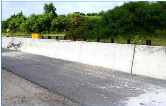
This research evaluated the MASH TL-4 performance of a 42-inch tall single slope concrete median barrier that was keyed into 1-inch thick asphalt and had a segment length of 40 feet. The barrier was evaluated by performing MASH Test 4-12 and it passed the MASH evaluation criteria. At the time of this research, the 40-ft segment length was the shortest barrier segment length crash tested for the single slope barrier with the 1-inch key-in.
