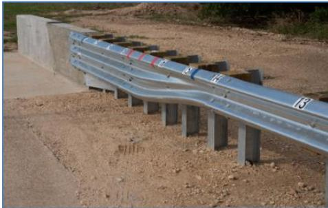
When roadways intersect with restrictive features, it becomes difficult to fit a transition system with proper length. This research project modeled and crash tested a shorter W-beam transition system design for MASH TL-3 evaluation criteria. Due to high ridedown acceleration during the crash test, the short transition did not satisfy the performance criteria for MASH Test 3-21 for transitions.
