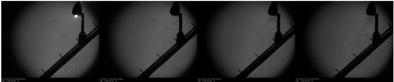
Figure 10: High-speed shadowgraph imaging sequence of shock tube in 3D printed O'Bellex model on a 40° inclined test slope showing both incident and reflected shock waves.
