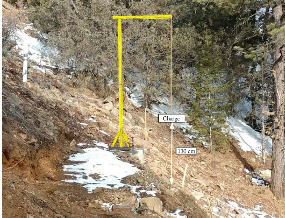
Figure 4: Explosive stand with horizontal charge orientation test setup with 130 cm standoff distance from the slope.
