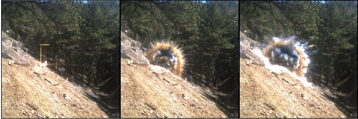
Figure 9: High-speed imaging sequence results of 8 lbs pentolite booster horizontal orientation (top) and 10 lbs ANFO vertical orientation (bottom).
