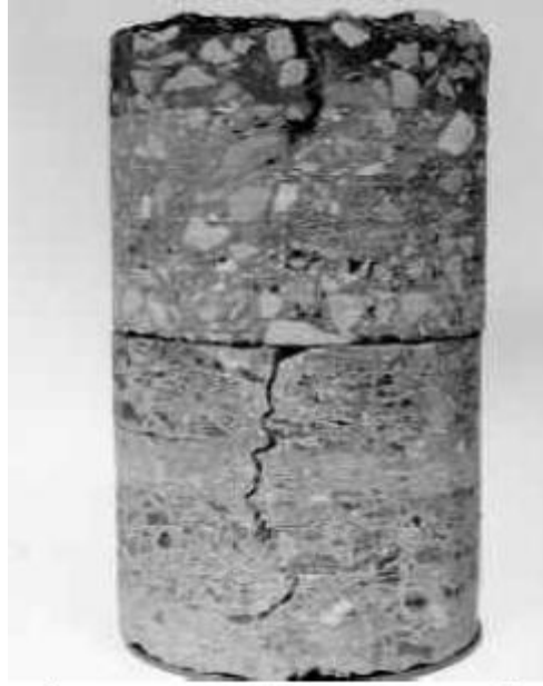
Figure 5.1. Core sample from recently initiated top-down crack in as-built AC/PCC (Nesnas and Nunn 2004).
