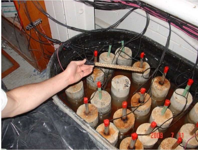
Figure 5. DC voltage through steel rod in the salt-water solution tank.
