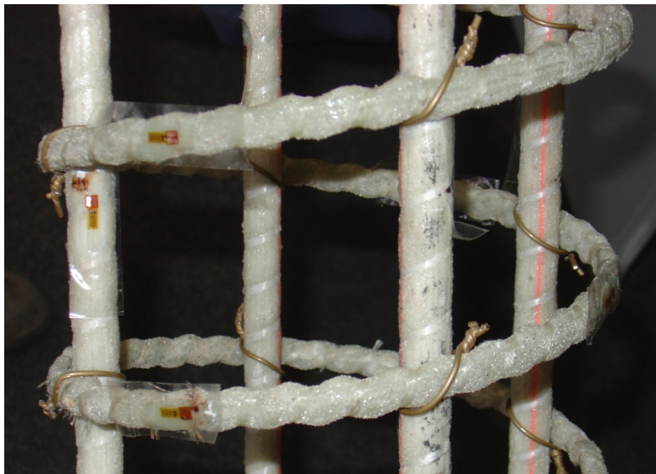
Figure 6. Nine strain gauges each (four on the longitudinal steel or GFRP bars and five on the internal steel or internal GFRP spirals) for control specimens.
