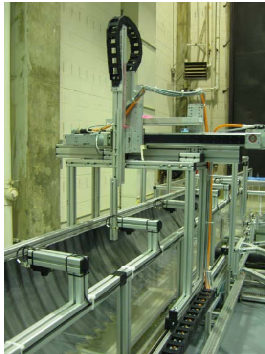
Figure 1: 2-dimensional robot that supports an Acoustic Doppler Velocity (ADV) probe
