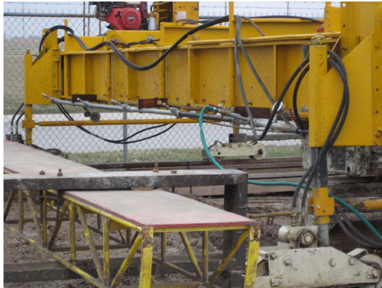
Fig. 5.36 Fogging system with solid pipe - did not deposit excessive water on the deck surface
