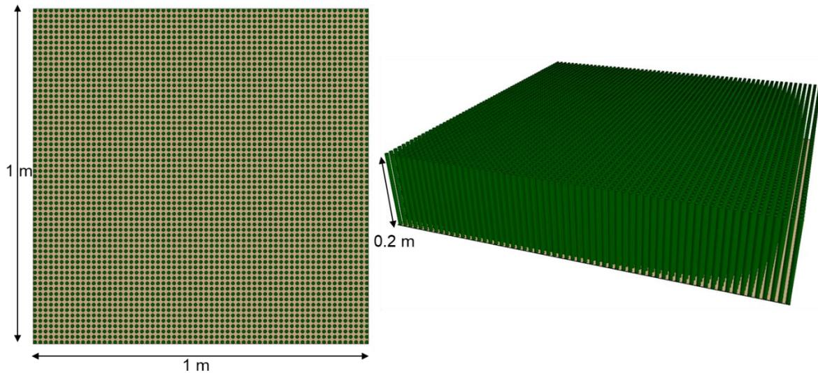
**Figure 2. Sketch of 4000 0.2-m-tall rigid cylinders in a uniform grid.**
