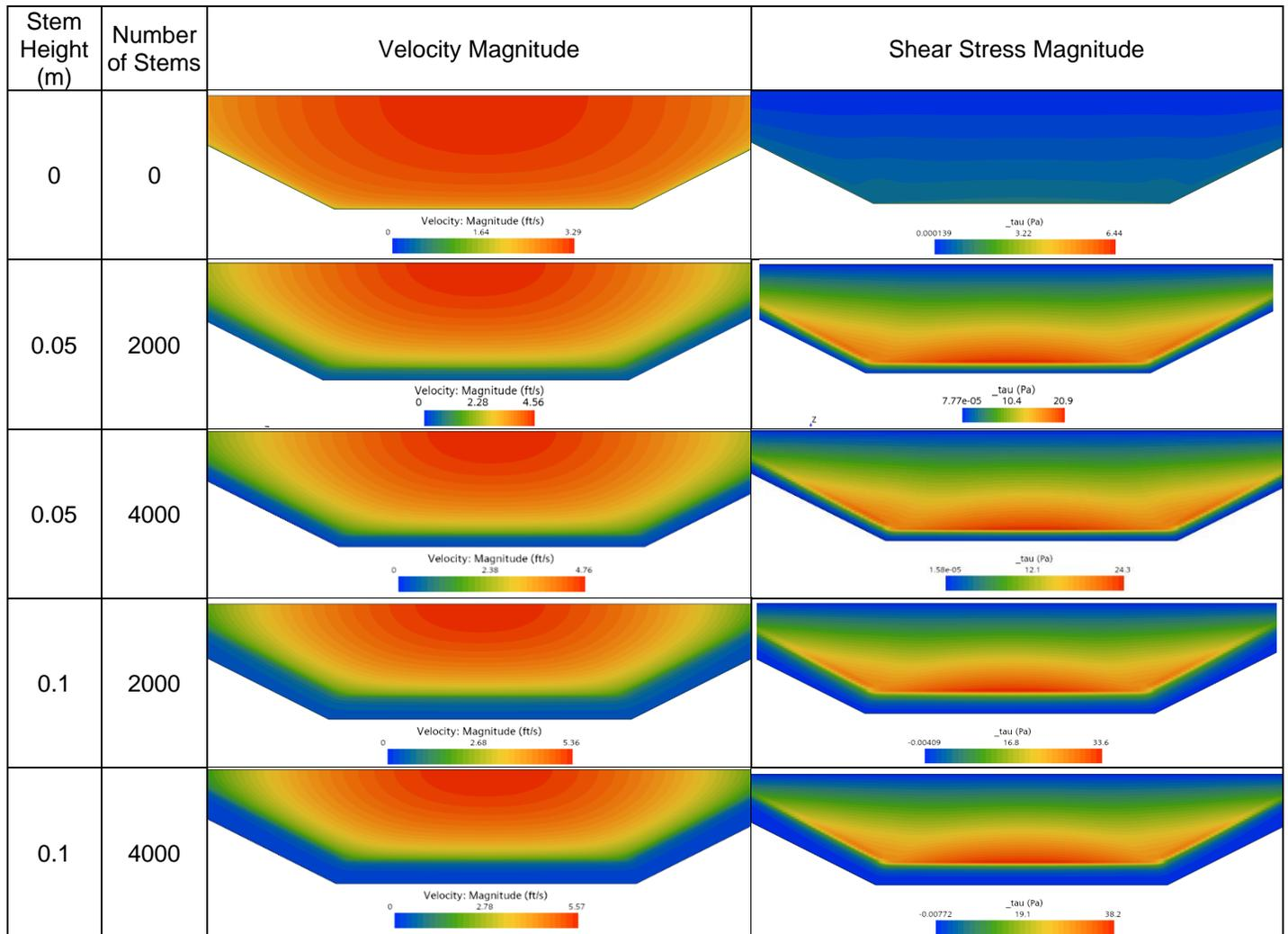
Figure 4. Velocity and shear stress magnitude contour plots on a cross-section through a ditch.
