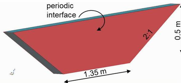
**Figure 3. Model of a thin strip of a roadside ditch.**
