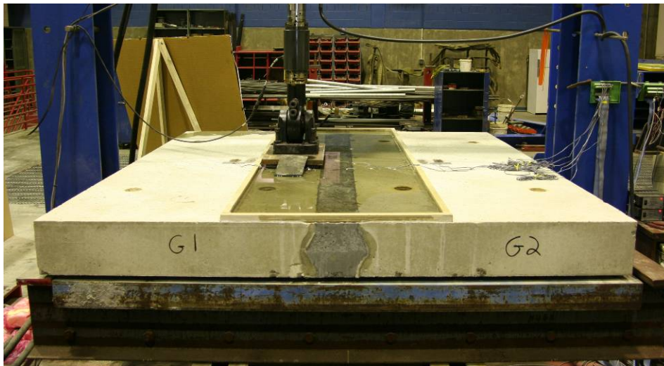
Figure 1. Photo of specimen G1-G2 in load frame during cyclic testing.
