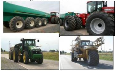
The testing was conducted at load levels of 0%, 25%, 50%, and 80% of the full capacity of each vehicle. There were 16 runs for each load level. Within those sixteen runs the wheel location (offset from the pavement edge), tire pressure, and speed of the vehicle were varied. Asphalt strain, pavement deformation and base vertical pressure measurements were collected. Data analysis of these measurements has been initiated.
