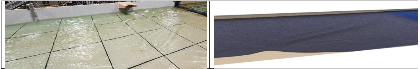
Figure 4. Standing wave at the pavement section downstream of the headbox.
