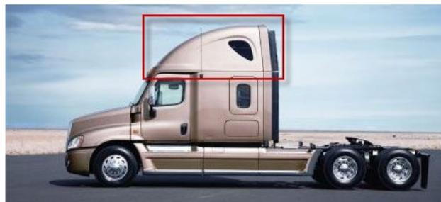
**Figure 9. Over-height vehicle selected for analysis (Aly & Hoffmann, 2022).**
