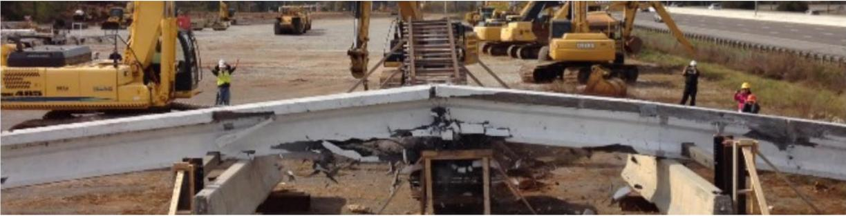
*Figure 39. PC girder after the impact test (Jing, 2017).*
