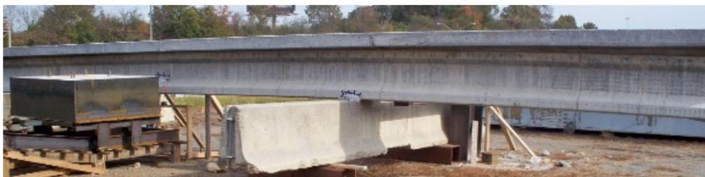
*Figure 38. Full-scale lateral impact test article with PC girder shown (Jing, 2017).*
