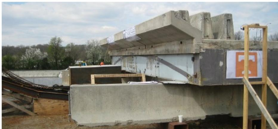
*Figure 37. Full-scale lateral impact test article with HCB shown (Jing, 2017).*
