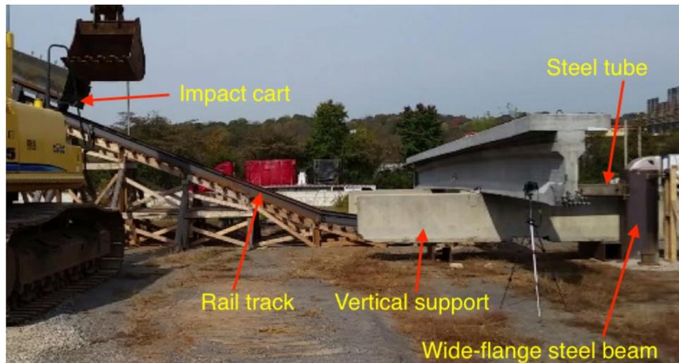
*Figure 36. Full-scale lateral impact test setup (Jing, 2017).*
