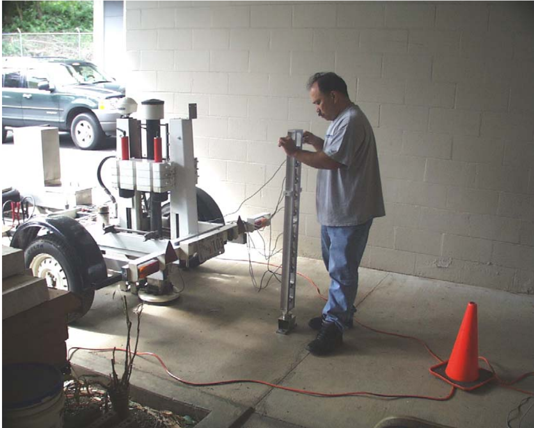
Figure 35. Photo. On site FWD calibration at Hawaii DOT Materials Lab.
