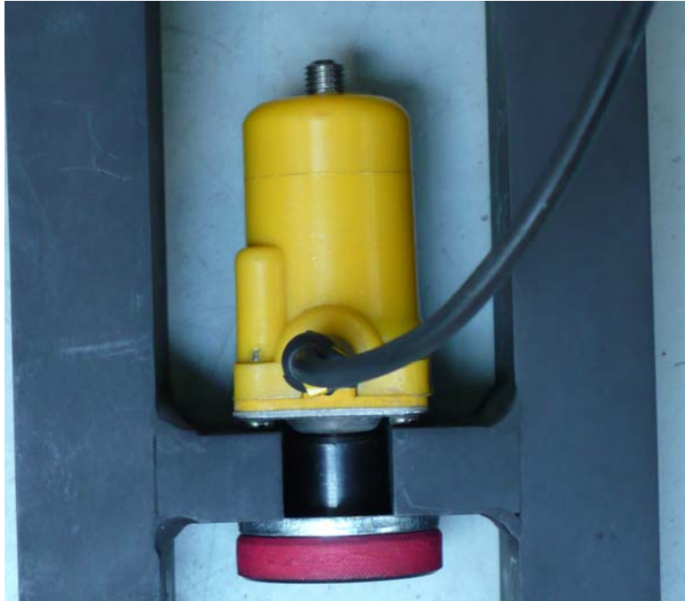
Figure 34. Photo. Attachment of a Carl Bro geophone in the stand.
