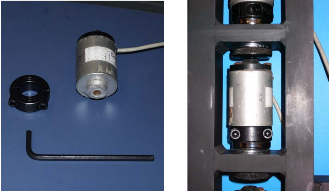
Figure 33. Photo. Attachment of a KUAB geophone in the stand.
