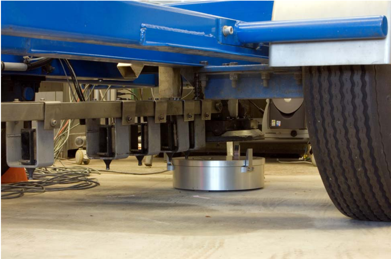
Figure 100. Photo. Reference load cell positioned under the FWD load plate.
