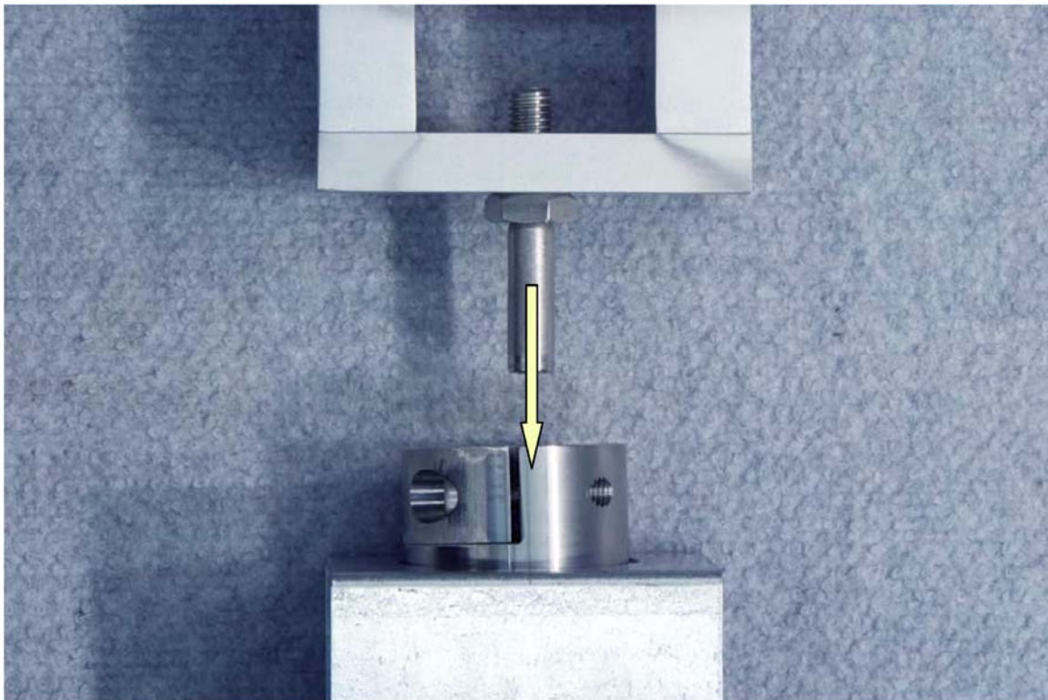
Figure 117. Photo. Coupling the calibration stand and ball joint anchor.
