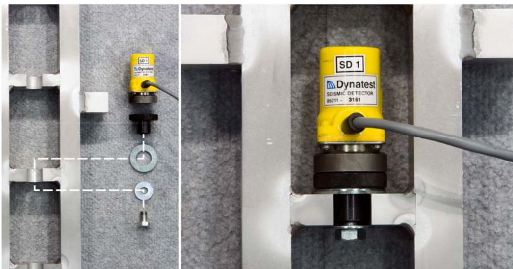
Figure 31. Photo. Attachment of a Dynatest geophone in the stand.
