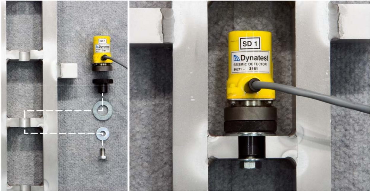
Figure 114. Photo. Attachment of a Dynatest geophone to the stand.
