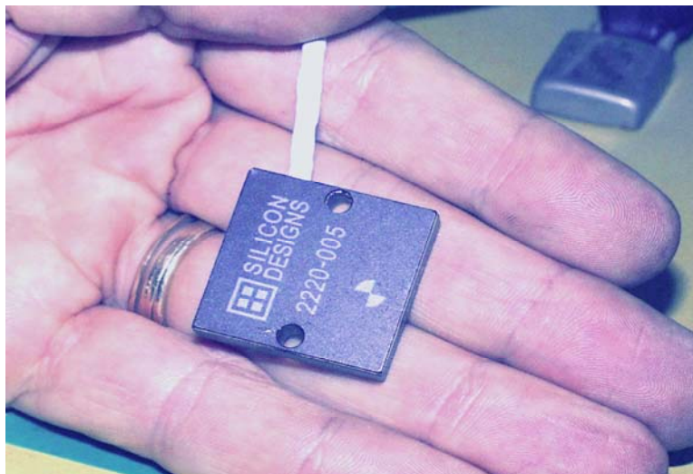
Figure 10. Photo. The Silicon Designs model 2220 accelerometer.
