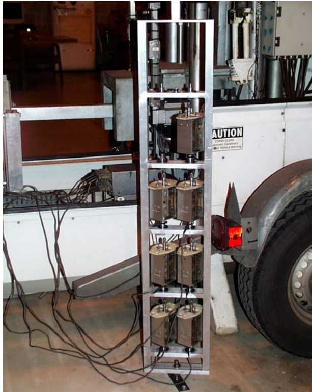
Figure 116. Photo. Seismometer stand with sensors attached.
