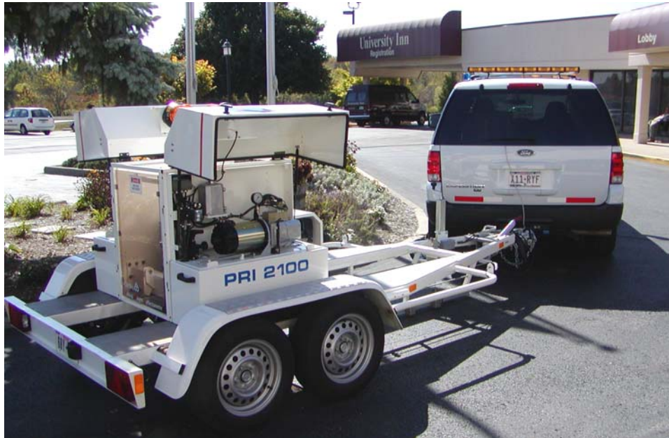
Figure 7. Photo. Carl Bro FWD
