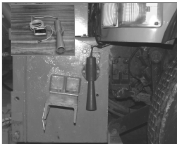
FIGURE 6.1 Typical sensor mounting.
