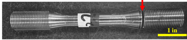
Figure 3-12 Low-cycle fatigue results of Ni-Ti-Co SMA at 50°C: (a) stress-strain curves, and (b) fractured sample.
