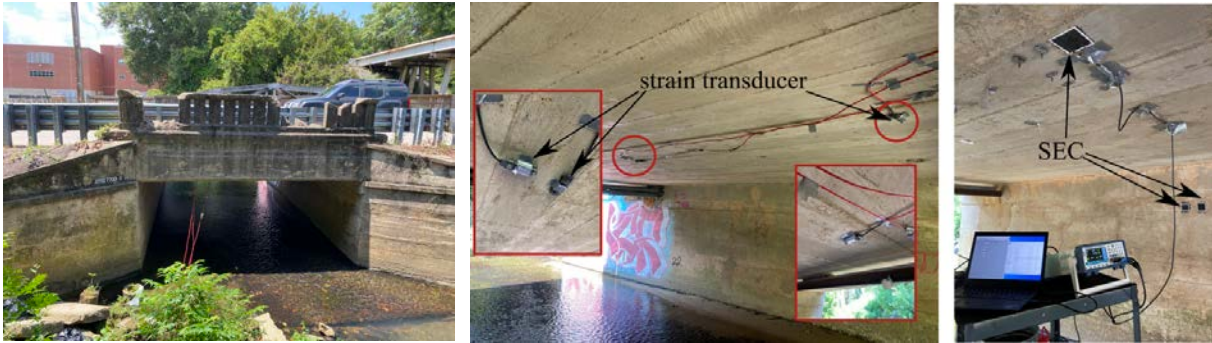
Figure: The bridge and the deployed sensors under the bridge.
