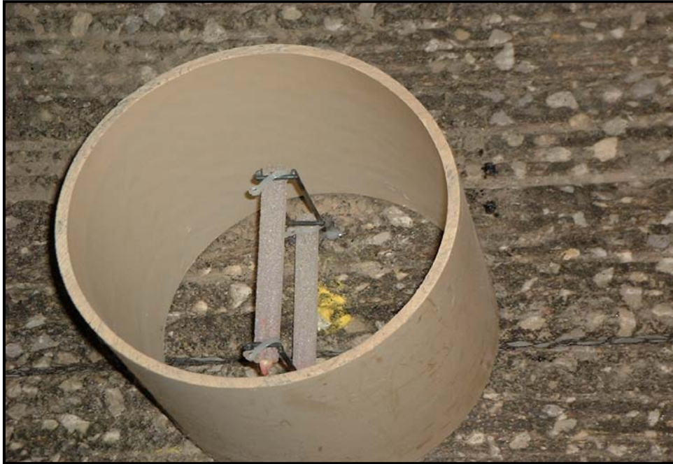
Figure 3.5: Strain Gages and Fixtures Setting
