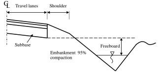
Figure 1. Typical section of a road with marked freeboard - clearance between the water free surface and bottom of the road subbase.
