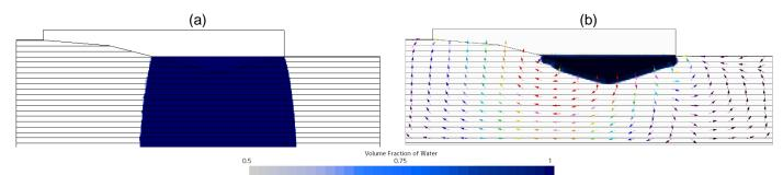
Figure 4. Water extent at 1 hour of simulated time in the model with (a) 40% porosity, and (b) 5% porosity.
