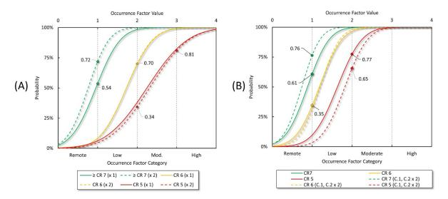
Figure 1. Results from back-casting (A) and Monte Carlo simulations (B) for bridge deck components.
