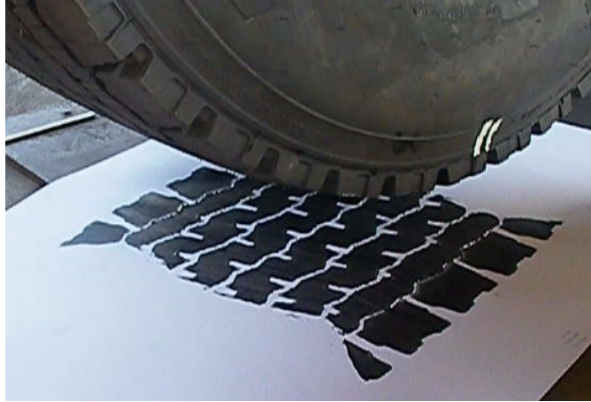
Figure 5. Photo. Measured Typical tire footprint for NG-WBT.
