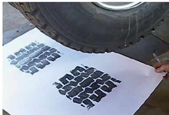
Figure 3. Photo. Measured Typical tire footprint for DTA.
