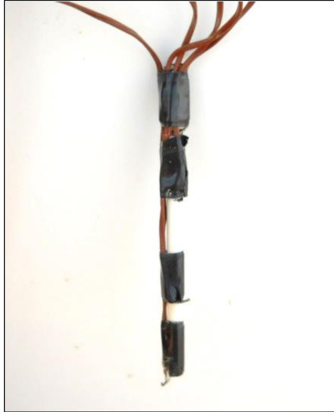
Figure 319. Photo. Thermocouple tree with five Type-K thermocouples on a plastic dowel.
