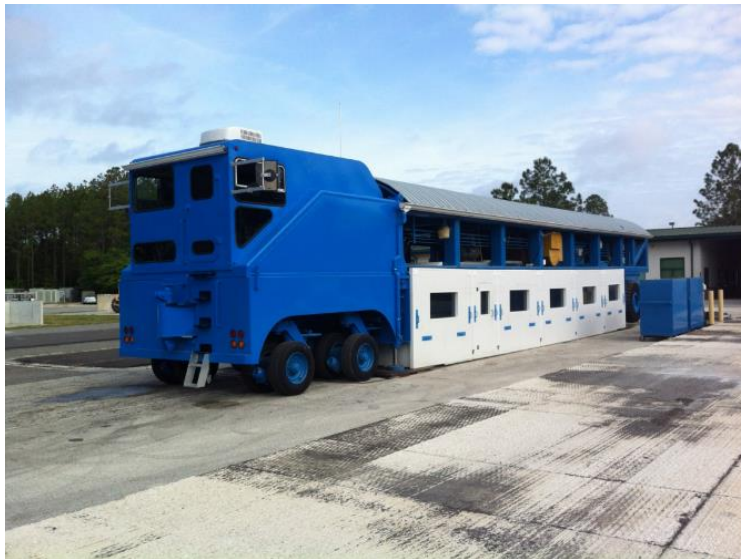
Figure 285. Photo. Insulated panels on HVS.
