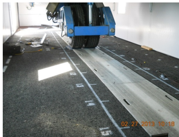
Figure 333. Photo. Heavy Vehicle Simulator (HVS) – inside view.
