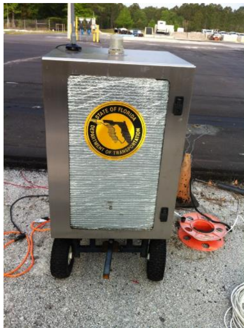
Figure 301. Photo. Mobile DAQ system - box.
