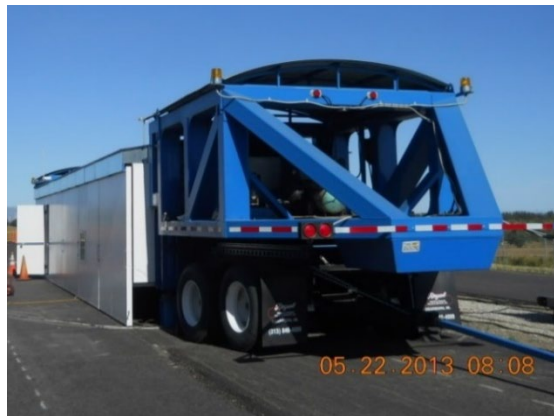
Figure 332. Photo. Heavy Vehicle Simulator (HVS) – outside view.
