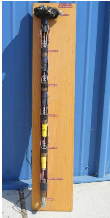
Figure 327. Photo. A model multi-depth deflectometer (MDD), showing five modules.
