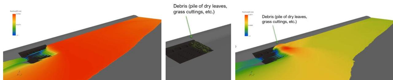
**Figure 4. Comparison of flow pattern for an unobstructed (left) and partially clogged (right) grate, for example conditions of longitudinal grade 0.01 ft/ft and upstream flow spread 4 ft.**
