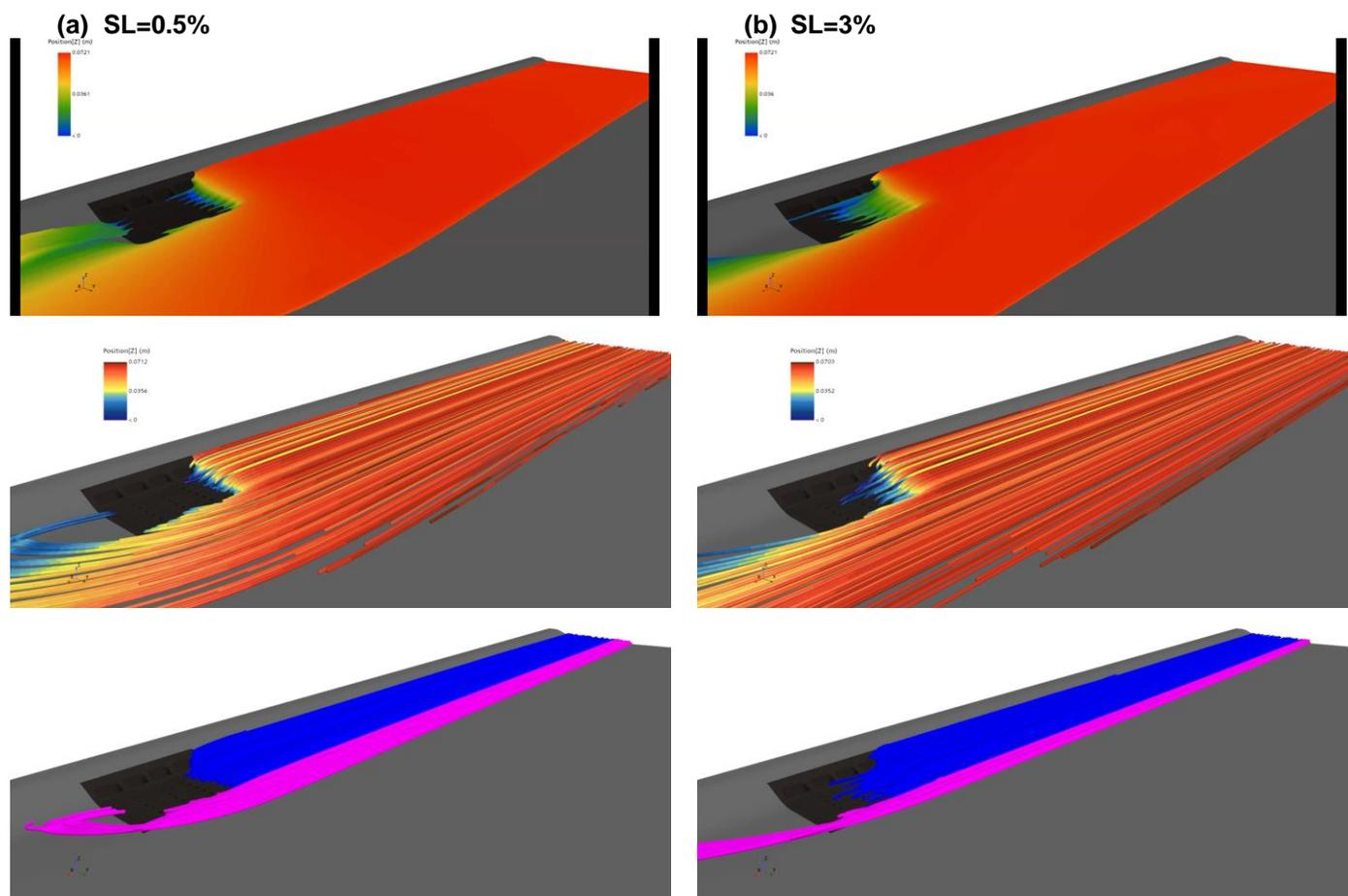
**Figure 5. Influence of the longitudinal grade on the flow interception. Example: upstream spread 5 ft, longitudinal grade (a) 0.5%, and (b) 3%. Top: water surface, center: velocity streamlines, bottom: streamlines intercepted by the front of the grate (blue) and intercepted by the side of the grate (pink).**
